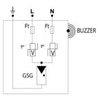
V: Varistor GSG: Specific gas tube Ft: Thermal fuse Buzzer: Audible disconnection indicator t\*: Thermal system disconnection
