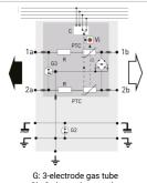
G: 3-electrode gas tube Gb: 2-electrode gas tube PTC: Thermal resistor R: Resistor D: Clamping diode Vi: Indicator
