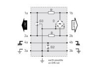
G: 3-electrode gas tube Gb: 2-electrode gas tube R: Resistor D: Clamping diode
